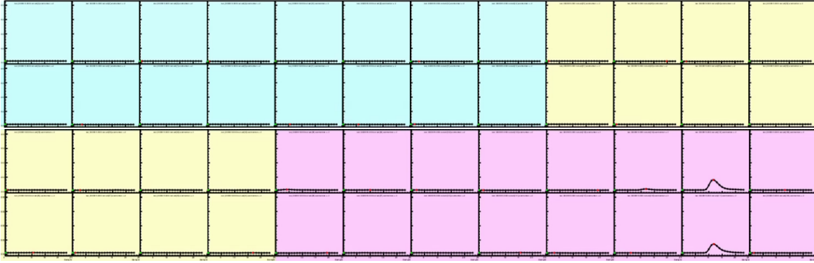
Figure 4: The signals from 48 towers in a sector for one hit are shown at the same time. The 48 towers are shown in two lines. The blue towers are the south part; the yellow towers are the middle part; and the red towers are the north part.
